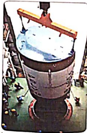
Integration of PSLV-C46 at MST - East Launch Pad
