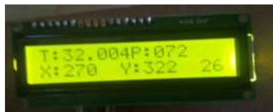
Fig10: Temperature, pulse rate, distance displayed in lcd
