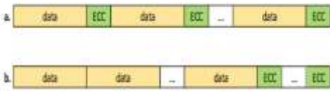
Fig. 2. (a) ECC bits stored alongside data bits. (b) ECC bits stored separately in memory (Separate Parity).
