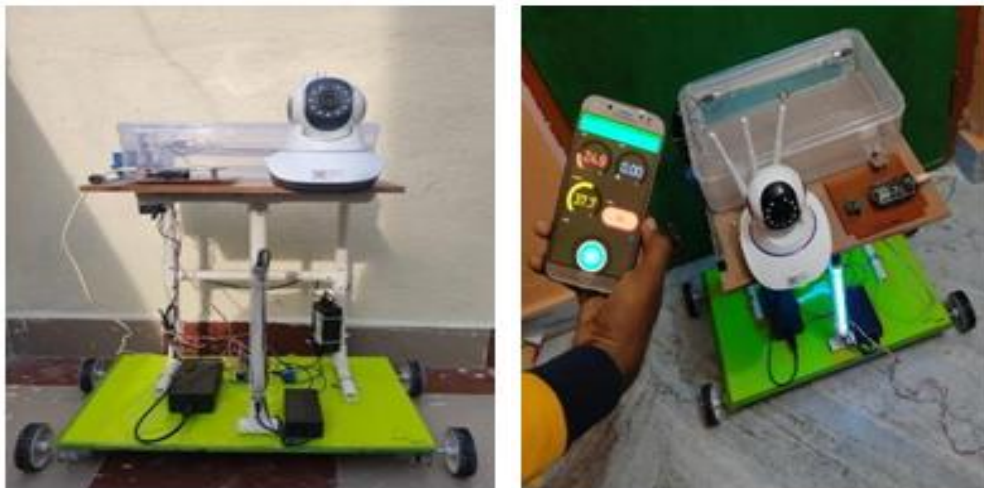
Figure:3 Hardware setup of smart nursing robot with uv lamps
