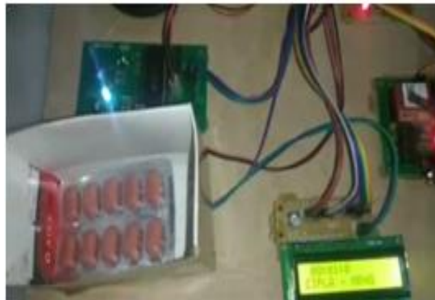
Figure 9: Figure showing LCD display indicating the time and Tablet to be taken by patient
