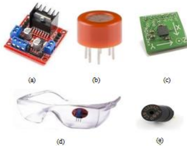
Figure 2 a) L298N Motor Driver, b) Alcohol Sensor, c) MEMS, d) Eye Blink Sensor and e). Buzzer
