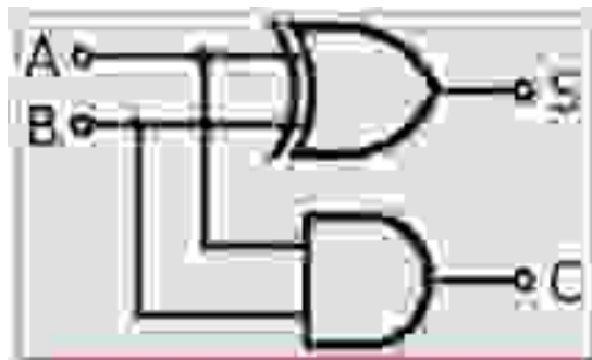
Fig: 2 Logic circuit of half adder
